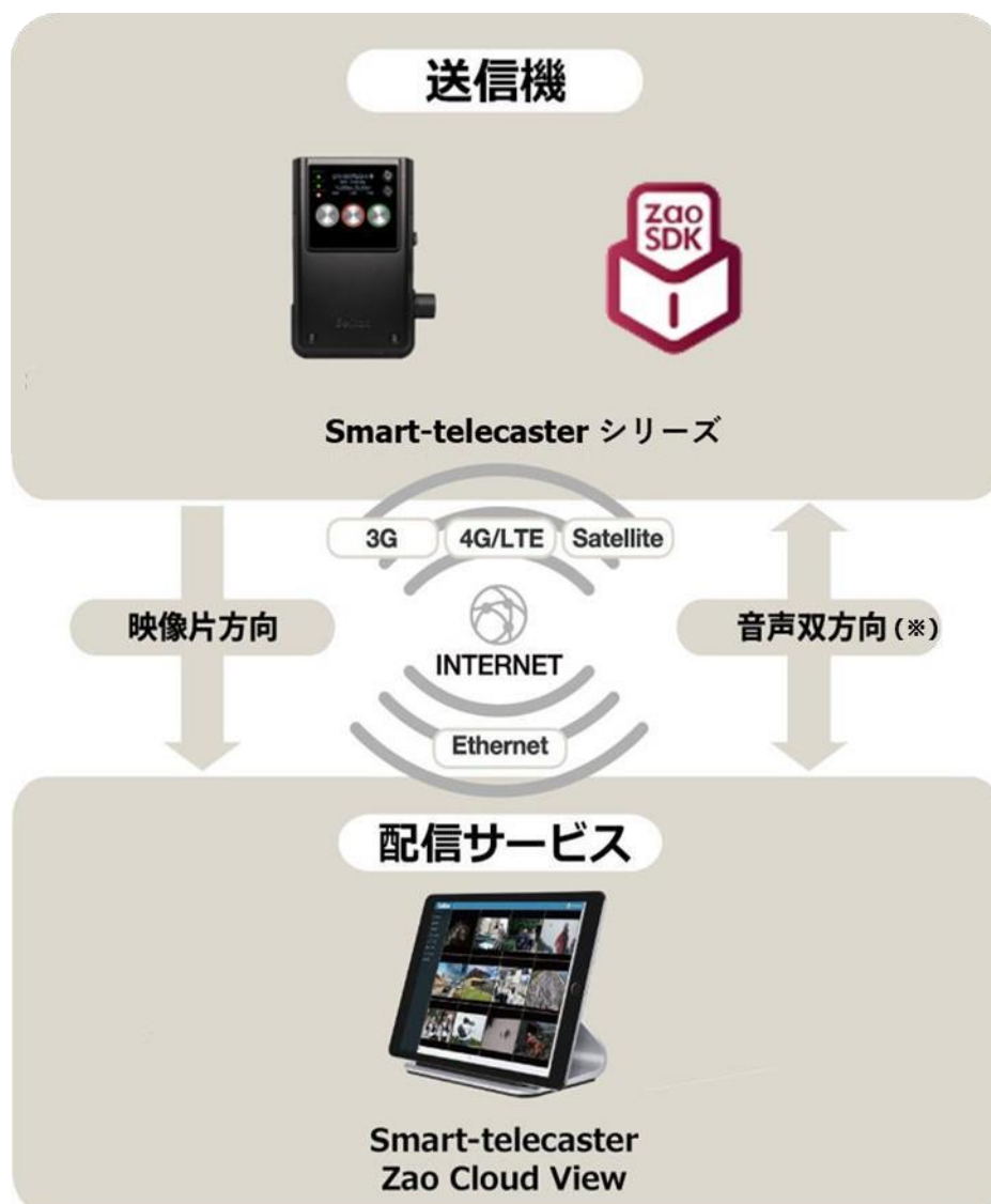
Figure 1 Overall system configuration
